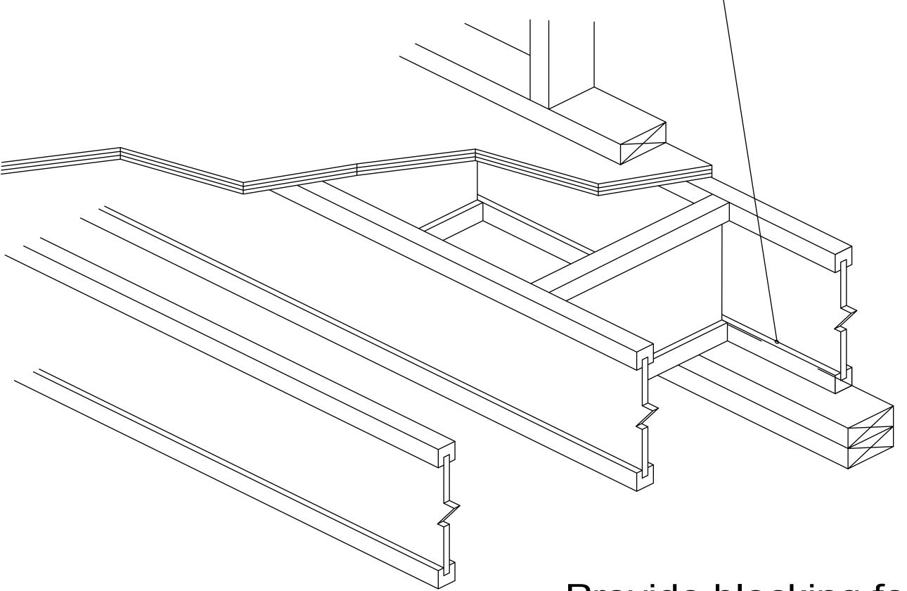
Provide blocking for lateral support as required. Use LP I-Joist, LP LVL, LP LSL, or LP Rim Board as blocking
