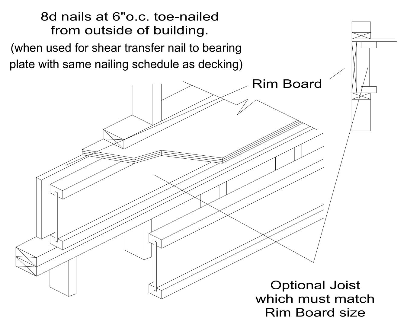
Provide blocking for lateral support as required. Use LP I-Joist, LP LVL, LP LSL, or LP Rim Board as blocking
