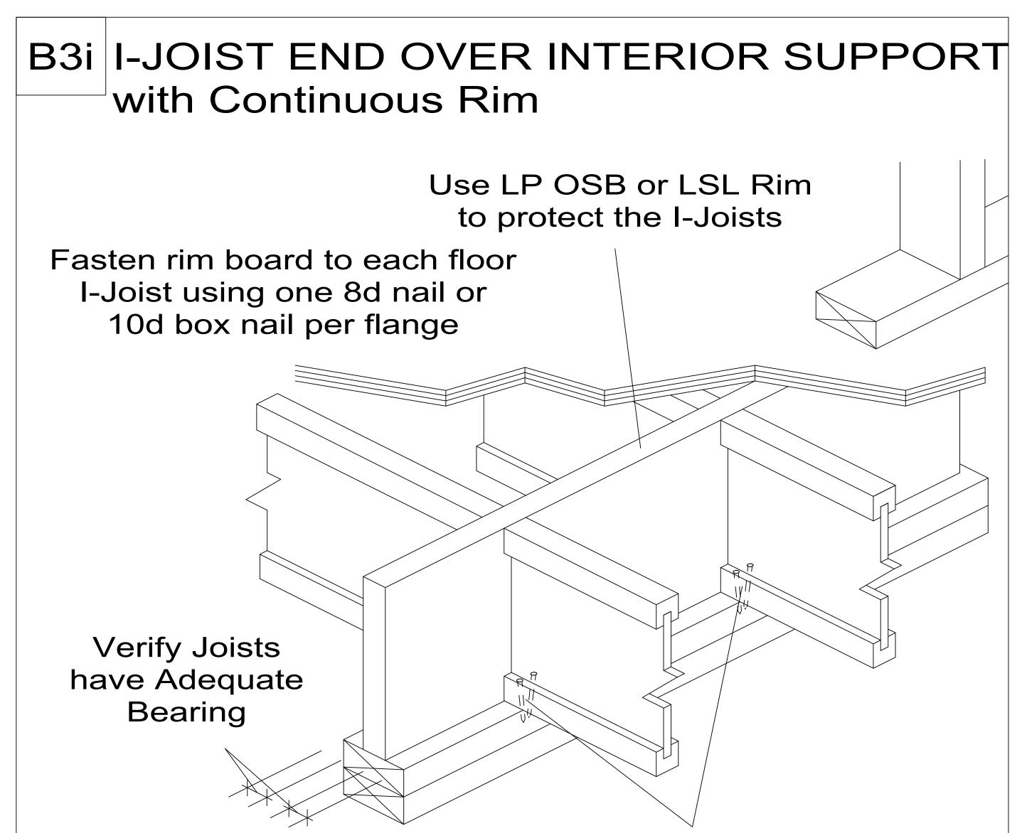
8d nail at 6" o.c. (when used for shear transfer nail to bearing plate with same nailing schedule as decking)
