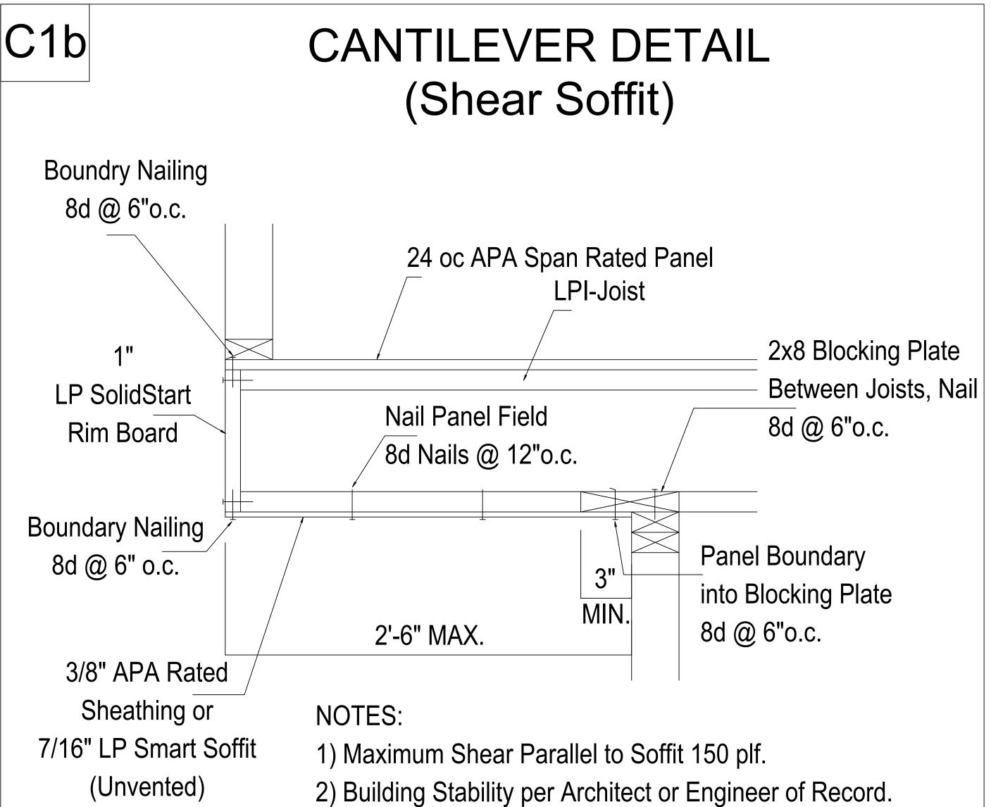
3) LPI-Joist to be Designed to Carry Wall Load
