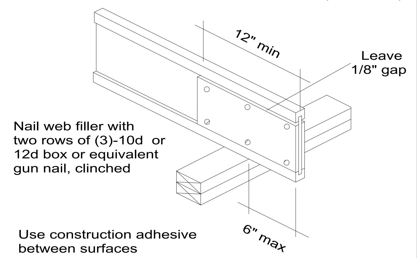
LP SolidStart Blocking panels are required at the bearing, but are not shown for clarity.
