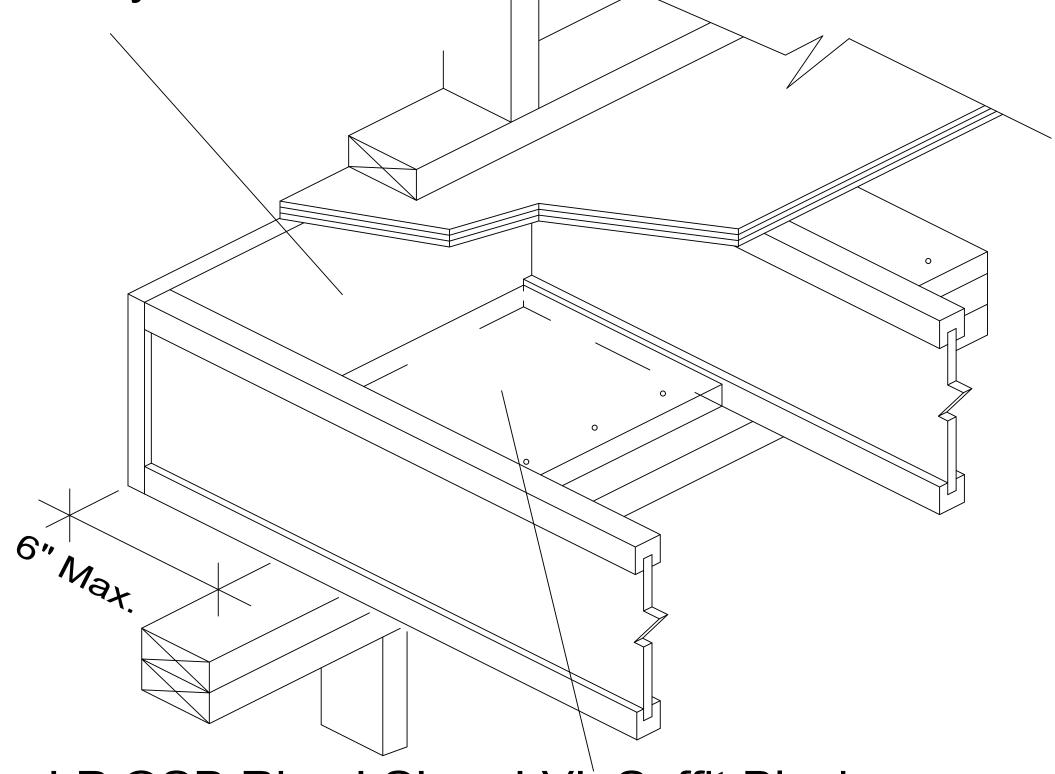
2x or LP OSB Rim, LSL or LVL Soffit Block. Block must extend from inside face of cantilever closure to inside face of the bearing wall. Attach to bearing wall as required by code.
