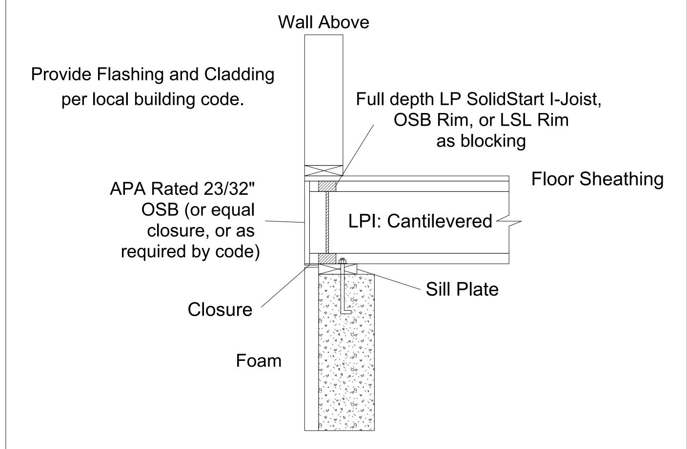
Verify Cantilever Capacity. No Cantilever Reinforcing is required when the full depth blocking (LPI, LSL, or OSB) is completely: under the wall above, and above the sill plate below. Designer is responsible for verifying that the blocking is capable of transfering all loads (both vertical and lateral).
