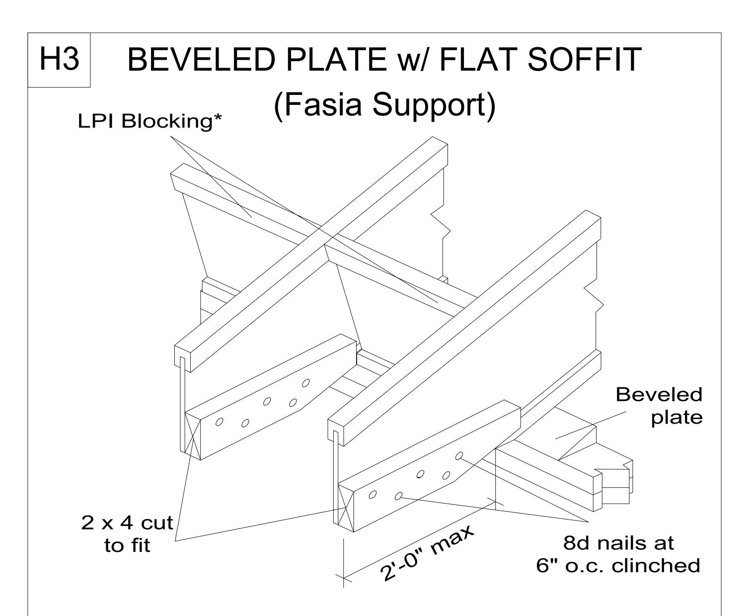
\* Lateral resistance shall be provided. Other methods of restraint, such as full depth LP® SolidStart® OSB Rim, LSL, or LVL may be substituted for the LPI blocking shown.
