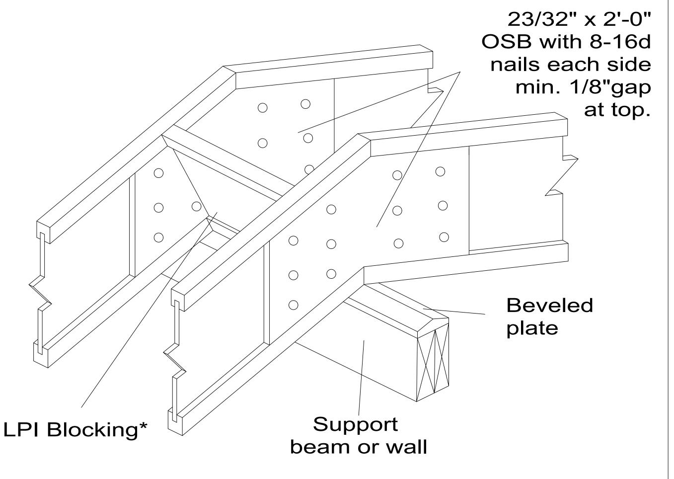
\* Lateral resistance shall be provided. Other methods of restraint, such as full depth LP SolidStart OSB Rim, LSL, or LVL may be substituted for the LPI blocking shown.
