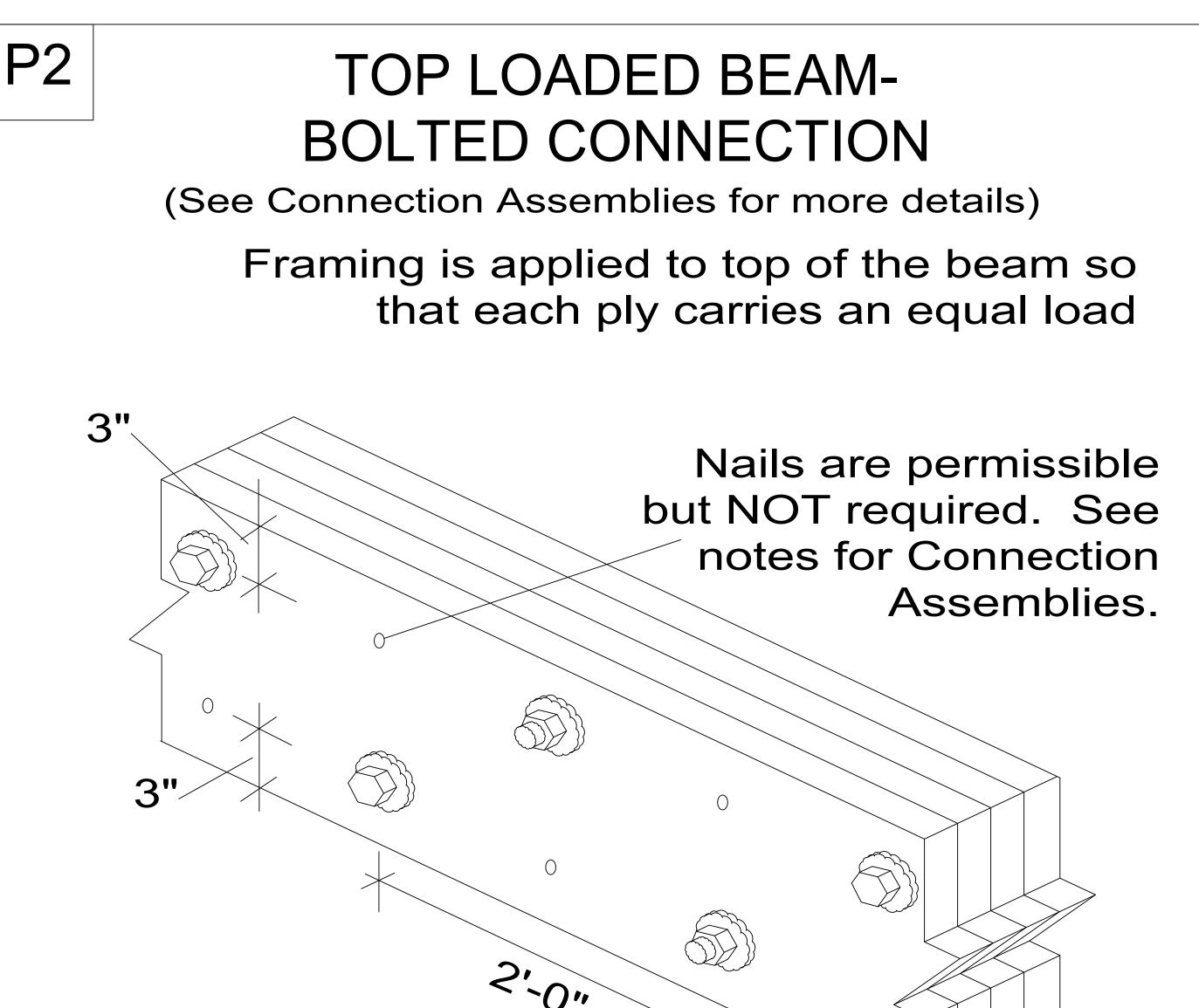
1/2" diameterASTM grade A-307(or better) bolts.Use washers on both faces.
