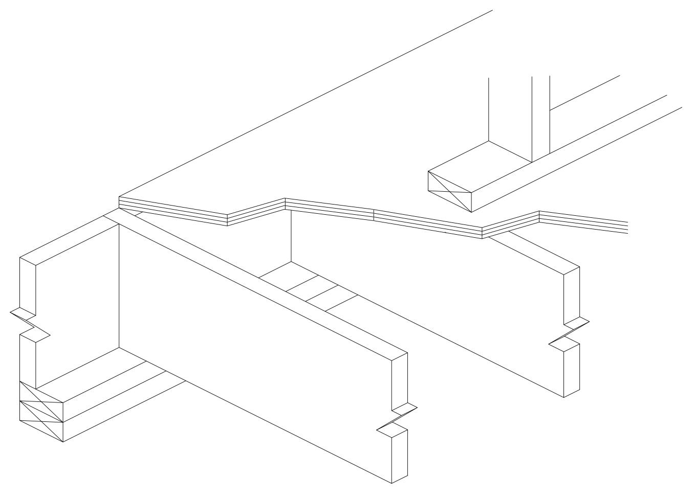
LP SolidStart LSL and LVL Joists shall be designed to carry all applied loads including walls from above that do not stack directly over the support.
