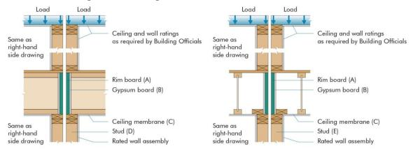
**Double Wall Configuration with No Load Transfer Base Assembly**
