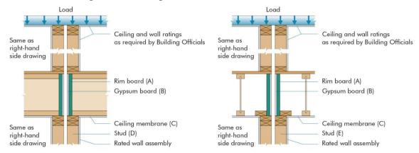
**Double Wall Configuration with Load Transfer Base Assembly**
